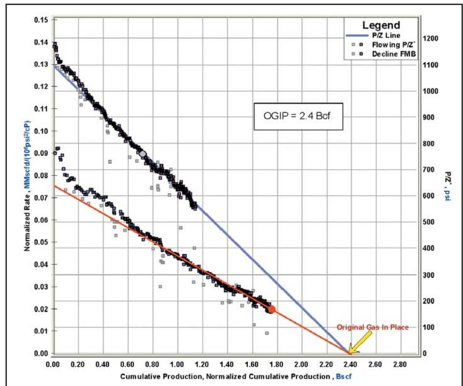
Figure 4 – Flowing material balance.
