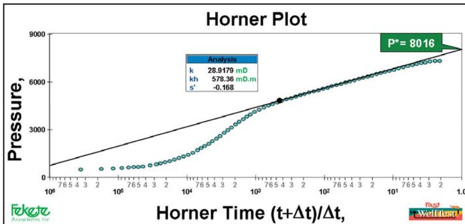
Figure 2. Semi-log (Horner) Plot of Build-up Data.
