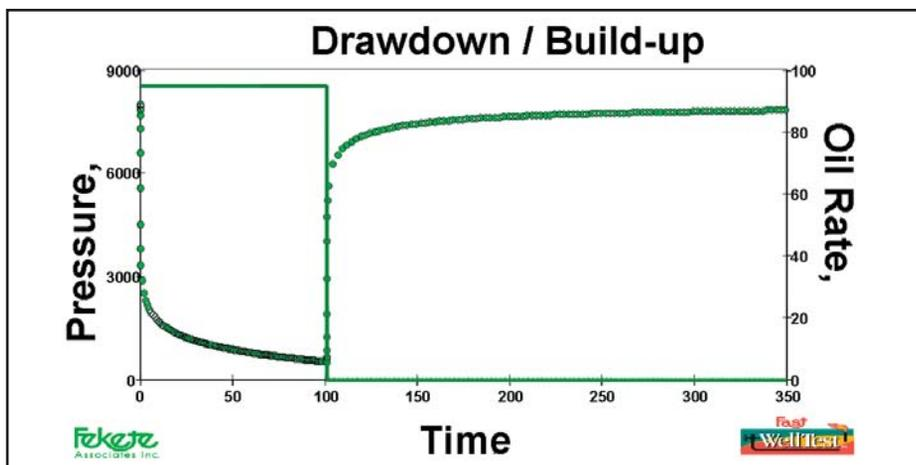
Figure 1. Drawdown and Build-up Test.
