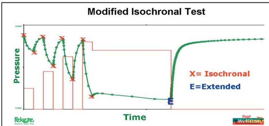
Figure 5. Modified Isochronal Test.
